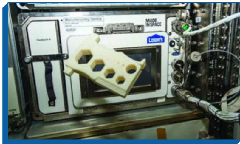
A printed product floats in front of the AMF on the ISS. (Image Credit: NASA)
